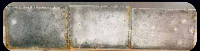
SLINTEC Coating: Coating formulated with graphene-based anti-corrosion additive
