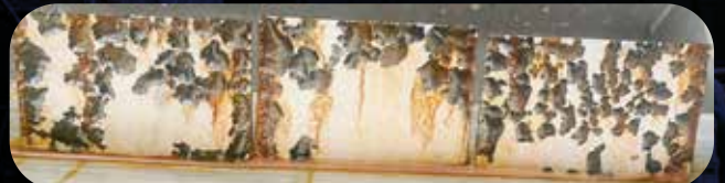
Control Sample: Base coating without any anti-corrosion additives
