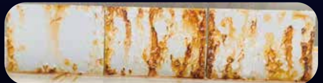
Commercial Coating: Coating enhanced with Zn-phosphate anti-corrosion additive
